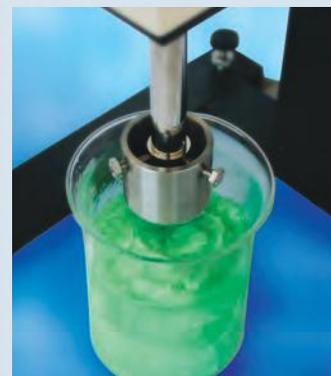
The PRO400 speeds through the homogenization of difficult samples. Shown here with the 02-37000 stainless steel deflector head (see page 8) attached to a 37mm generator for enhanced sample motion.
